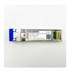
Huawei Optical Transceiver, TSFP+, Extended C Band, 9.95~11.3Gbps with CDR, -1dBm~3dBm, -16dBm, LC, SMF, 80km 34060852
