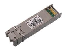
IBM 46C9246 46C9297 10GB SFP+ SR optical transceiver 46C9246
