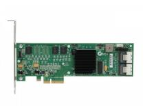
Broadcom LSI 8708ELP LSI00141 PCI Express x4 LSISAS1078 8 Internal 3Gb/s SAS/SATA Ports RAID On Chip Adapter 8708ELP
