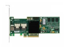
Broadcom LSI 8708EM2 LSI00187 PCI Express x8 LSISAS1078 8 Internal 3Gb/s SAS/SATA Ports RAID On Chip Adapter 8708EM2
