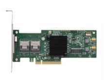
Broadcom LSI 9240-8i LSI00200 PCIe 2.0 x8 SAS2008 8 Internal Ports MegaRAID 6Gb/s SATA+SAS RAID Controller 9240-8i
