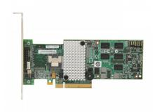
Broadcom LSI 9260-4i LSI00197 PCIe 2.0 x8 SAS2108 4 Internal Ports MegaRAID 6Gb/s SATA and SAS RAID Controller 9260-4i
