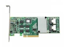
Broadcom LSI 9261-8i LSI00212 PCIe 2.0 x8 LSISAS2108 8 Internal Ports 6Gb/s SATA SAS RAID Controller 9261-8i
