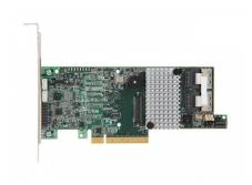
Broadcom LSI 9271-8i LSI00330 PCIe 3.0 x8 LSISAS2208 8 Internal Ports 6Gb/s SATA+SAS RAID Controller 9271-8i
