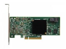
Broadcom LSI 9300-4i H5-25473-00 LSI00346 PCIe 3.0 x8 SAS3004 4 Internal Ports 12Gb/s SAS Host Bus Adapter 9300-4i
