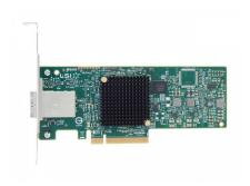
Broadcom LSI 9300-8e H5-25460-00 LSI00343 PCIe 3.0 x8 SAS3008 8 External Ports 12Gb/s SAS Host Bus Adapter 9300-8e
