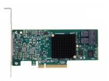
Broadcom LSI 9300-8i LSI00344 PCIe 3.0 x8 SAS3008 8 Internal Ports 12Gb/s SAS Host Bus Adapter 9300-8i
