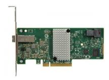
Broadcom LSI 9311-4i4e SAS3008-4I4E PCIe 3.0 x8 SAS3008 Fusion-MPT 4 Internal & 4 External Ports 12Gb/s SAS Host Bus Adapter
