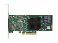
Broadcom LSI 9341-8i 05-26106-00 LSI00407 PCIe 3.0 x8 SAS3008 8 Internal Ports MegaRAID SATA+SAS RAID Controller 9341-8i
