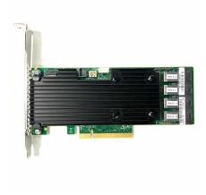
Broadcom LSI 9361-16i 05-25708-00 PCIe 3.0 x8 SAS3316 16 Internal Ports 12 Gb/s SATA + SAS RAID Controller 9361-16i
