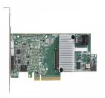
Broadcom LSI 9361-4i LSI00415 PCIe 3.0 x8 SAS3108 4 Internal Ports MegaRAID SATA+SAS RAID Controller 9361-4i
