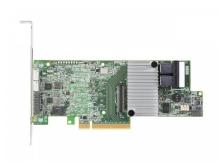
Broadcom LSI 9361-8i LSI00417 PCIe 3.0 x8 SAS3108 8 Internal Ports MegaRAID SATA+SAS RAID Controller 9361-8i
