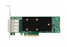
Broadcom LSI 9400-16e 05-50013-00 PCIe 3.1 x8 SAS3416 16 External Ports Tri-Mode Storage Adapter 9400-16e
