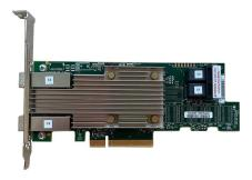
Broadcom LSI 9400-8i8e 05-50031-02 PCIe 3.1 x8 SAS3516 8 Internal & 8 External Ports Tri-Mode Storage Adapter 9400-8i8e
