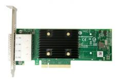
Broadcom LSI 9500-16e 05-50075-00 PCIe 4.0 x8 SAS3816 16 External Ports 12Gb/s SAS, 6Gb/s SATA, Gen 4.0 PCIe(NVMe) Tri-Mode HBA
