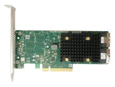
Broadcom LSI 9500-16i 05-50134-00 PCIe 4.0 x8 SAS3816 16 Internal Ports 12Gb/s SAS, 6Gb/s SATA, Gen 4.0 PCIe(NVMe) Tri-Mode HBA
