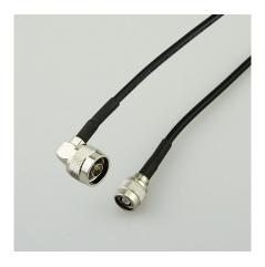
Cisco AIR-CAB020LL-R-N 20-ft low-loss cable, one RP-TNC plug, one 90-degree N male connector AIR-CAB020LL-R-N
