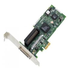
Adaptec ASC-29320LPE 2248700-R PCIe x1 Single-Channel Ultra320 SCSI Host Adapter
