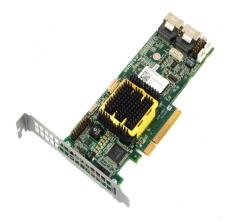
Adaptec ASR-5805 2244300-R 3Gb/s 8-port Internal SAS/SATA RAID Controller with 512MB Cache ASR-5805
