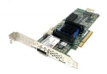
Adaptec ASR-6445 2270200-R 6Gb/s 8-port (4 internal/4 external) PCIe Gen 2 x8 SAS SATA RAID Controller ASR-6445
