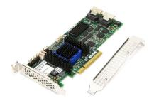
Adaptec ASR-6805 2270100-R 6Gb/s 8-port Internal PCIe Gen 2 x8 SAS SATA RAID Controller ASR-6805
