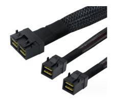
Internal HD Mini SAS SFF-8643 8i 72P to 2x HD Mini SAS SFF-8643 4i Breakout Cable CAB-8643i8-2x8643i4
