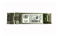
Cisco CWDM-SFP10G-1490 CWDM 1490-nm SFP+; 10 Gigabit Ethernet
