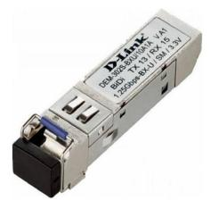
D-Link DEM-302S-BXU SFP Transceiver 1 Port 1000Base-BX for SMF, power supply 3.3V (up to 2km), WDM (TX: 1310nm, RX: 1550nm)
