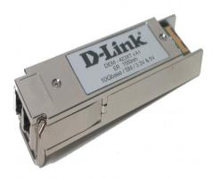
D-Link DEM-423XT 10.5 Gbps 10GBASE-ER 1550nm Single Mode 40km XFP Transceiver DEM-423XT
