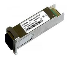
D-Link DEM-424XT 10GBASE-ZR SMF 1550nm 80km XFP Transceiver
