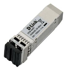
D-Link DEM-434XT-DD 10GBase-ZR SFP+ Transceiver (SMF, 1550nm, 80km, LC, DOM) DEM-434XT-DD
