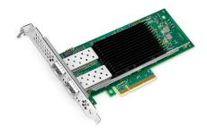
Intel E810XXVDA2G1P5 25 Gigabit Dual-Port PCIe 4.0 x8 Ethernet Network Adapter
