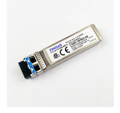
Finisar FTLX1370W4BTL 10G CPRI Wireless 1.4km Industrial Temperature SFP+ Optical Transceiver
