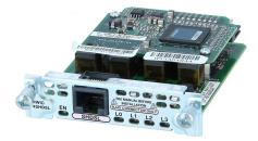
Cisco HWIC-4SHDSL 4-pair G.shdsl HWIC with IMA support HWIC-4SHDSL
