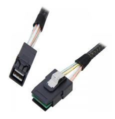
LSI LSI00400 SFF8643 to SFF8087 (mini SAS HD to mini SAS) 0.6m Internal Cable LSI00400
