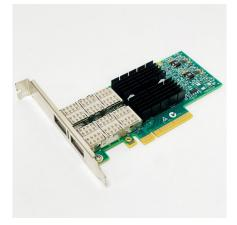
Mellanox MCX354A-FCBT ConnectX-3 VPI Adapter Card, Dual FDR 56Gb/s or 40/56GbE QSFP Port, PCIe 3.0 x8 8GT/s MCX354A-FCBT
