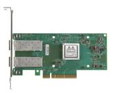
Mellanox MCX512A-ACUT ConnectX-5 EN network interface card, 10/25GbE dual-port SFP28, PCIe3.0 x8, UEFI Enabled (x86/ARM), tall bracket
