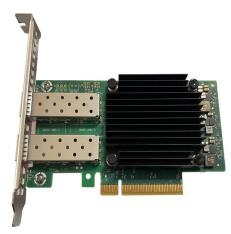
Mellanox MCX621102AN-ADAT ConnectX-6 Dx EN adapter card, 25GbE, Dual-port SFP28, PCIe 4.0 x8, No Crypto, Tall Bracket
