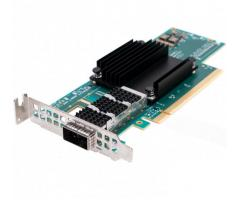
Mellanox MCX653105A-ECAT-SP ConnectX-6 VPI adapter card, 100Gb/s (HDR100, EDR IB and 100GbE), single-port QSFP56, PCIe3.0/4.0 x16, tall bracket, single pack
