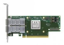
Mellanox MCX653106A-HDAT ConnectX-6 VPI adapter card, HDR IB (200Gb/s) and 200GbE, dual-port QSFP56, PCIe4.0 x16, tall bracket
