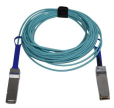
Mellanox MFA1A00-E010 active fiber cable, IB EDR, up to 100Gb/s, QSFP, LSZH, 10m
