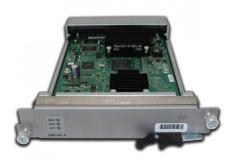
Cisco N9K-SC-A System Controller for Nexus 9500
