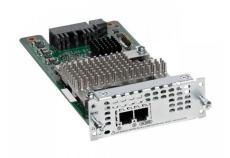
Cisco NIM-2FXS 2-Port Network Interface Module - FXS. FXS-E and DID
