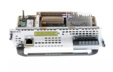
Cisco NM-AIR-WLC6-K9 Wireless LAN Controller Network Module for up to 6 lightweight access points
