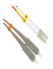
0.5m (1.6ft) 62.5/125 OM1 LC to SC UPC Duplex Multimode Fiber Optic Patch Cable OM1-LC-SC-D05M
