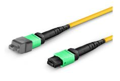
Single Mode MPO-16 Female to MPO-16 Female Trunk Cable, 16 Fiber, 9/125 OS2, Type B, LSZH, 1m (3.3ft)
