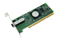
Genuine Qlogic QLA2460-CK PCI-X Single-port 4Gb Fibre Channel Host Bus Adapter QLA2460
