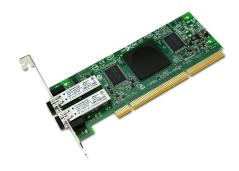
Genuine Qlogic QLA2462-CK PCI-X Dual-port 4Gb Fibre Channel Host Bus Adapter QLA2462
