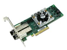
Genuine Qlogic QLE2672-CK PCIe 3.0 x8 Dual-port 16GFC SR-Optic Low Profile 16Gb Fibre Channel Adapter QLE2672
