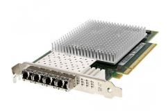
Genuine Qlogic QLE2764-SR-CK PCIe 3.0 x16 Quad-port 32GFC SR-Optic SFP+ 32Gb Fibre Channel Adapter QLE2764
